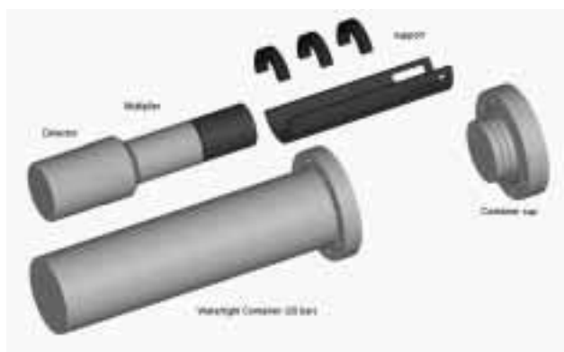
Fig. 2: The watertight cylindrical casing, which houses the sensor, the photomultiplier and the appropriate sled.
