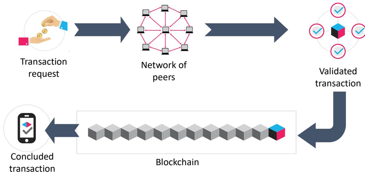
Figure 2. Basic flow of a blockchain transaction
