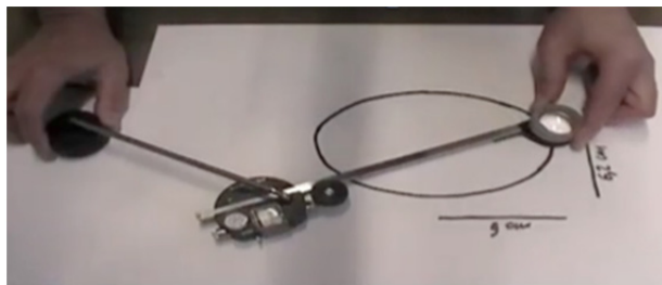
Figure 2. The Amsler planimeter
