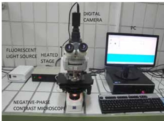
Fig. 1. Equipment for Computer Assisted Sperm Analysis.
