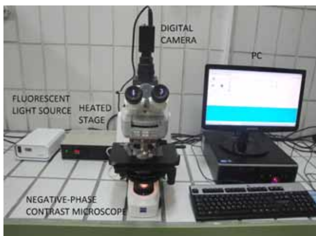
Fig. 1. Equipment for Computer Assisted Sperm Analysis.
