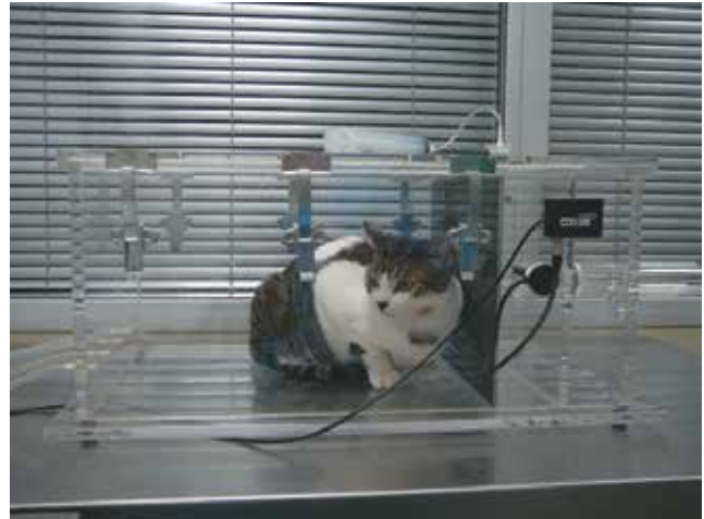
Figure 1. Cat placed into a plethysmography chamber connected to commercial software, used to analyse the respiratory patterns. The chamber is placed in a quiet room with calibrated temperature and humidity, and cats are acclimated to the chamber for 5 minutes after which data are recorded for a period of 12 minutes.
