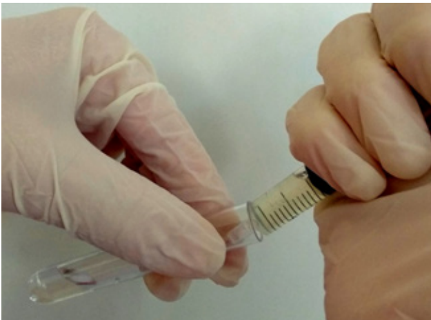
Figure 3. Add equal amount of urine in the tube by layering the urine sample above the nitric acid, caution should be given in order not to mix the samples.
