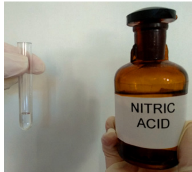
Figure 2. Put a small amount of nitric acid (approximately 1ml) in the tube.
