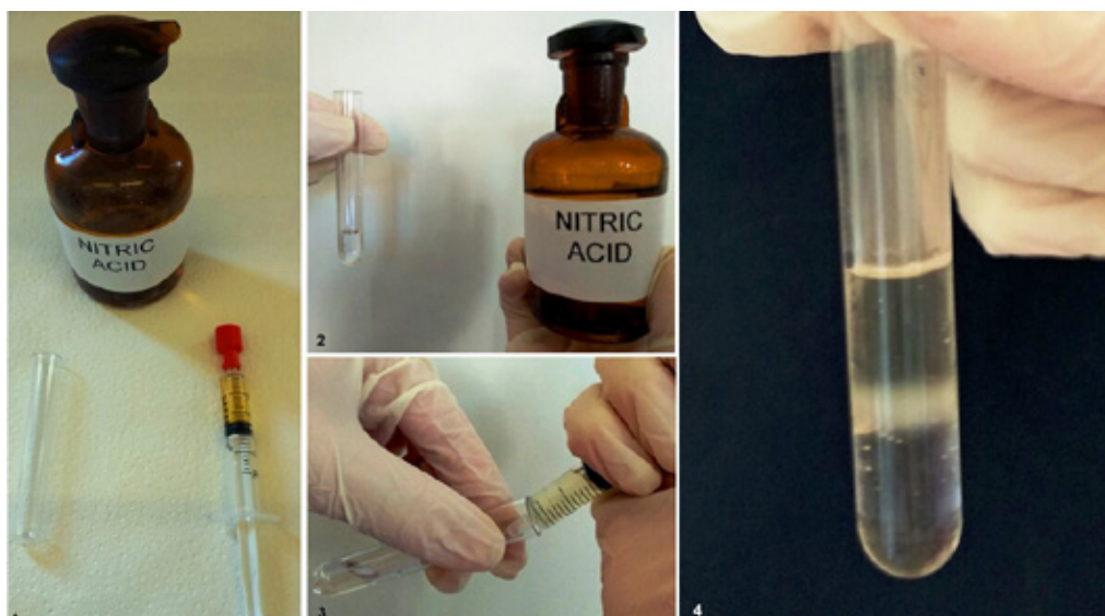
Figures 1-4. Procedure of Heller's reaction test.
