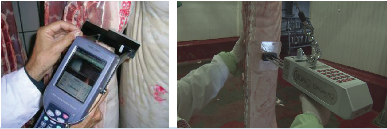
Picture 1. Measurement points using Optiscan-TP and Optigrade-MCP
