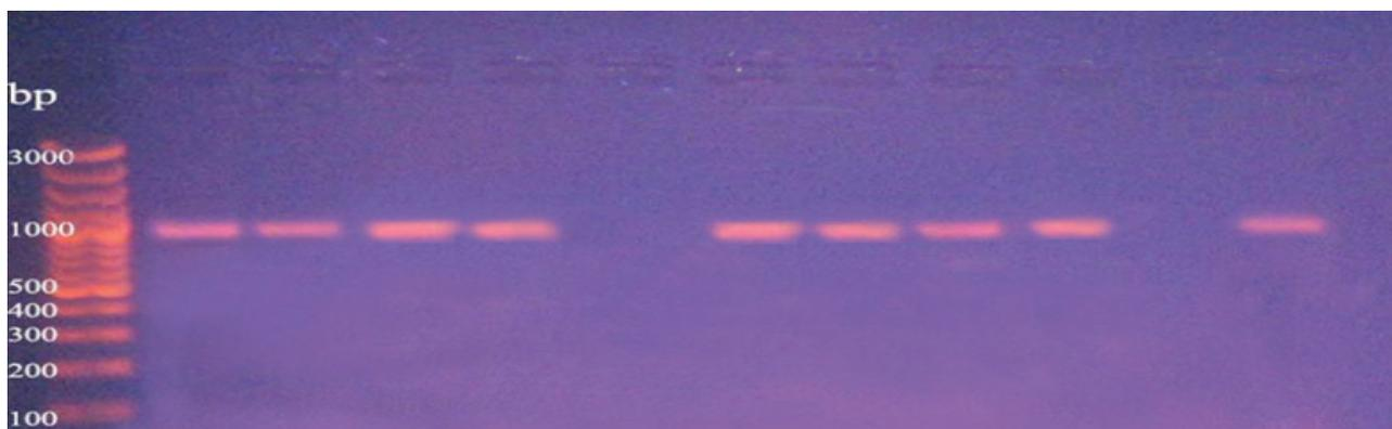
**Fig. 1.** Typical amplicon of the gene 16S rRNA product of *Pseudomonas aeruginosa* isolates on agarose gel electrophoresis (1.5%) showing the Lane (M) DNA marker (3000 bp), Lane (1-10) represent positive isolates
