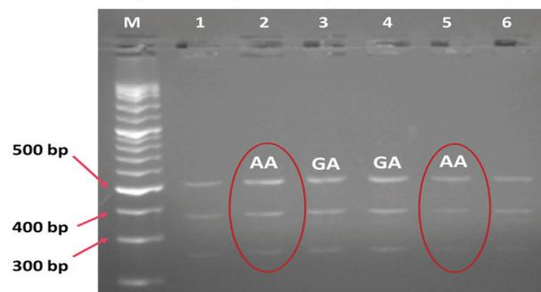
**Figure 1.** Agarose gel electrophoresis results of *AA-NAT* gene. The M symbolizes the 100 bp ladder molecular weight markers. Line 1 of KM belongs to GG genotype with the 371, 333, and 285 bp fragments. The Line 4 of KM; Lines 2 and 5 of Kivircik sheep exhibit AA genotype (516, 371, and 285 bp). Moreover, Line 2, 3, 5, and 6 refer to the heterozygote GA genotype (516, 371, 333, and 285 bp) for KM. (The 183 bp fragment is not visible).
