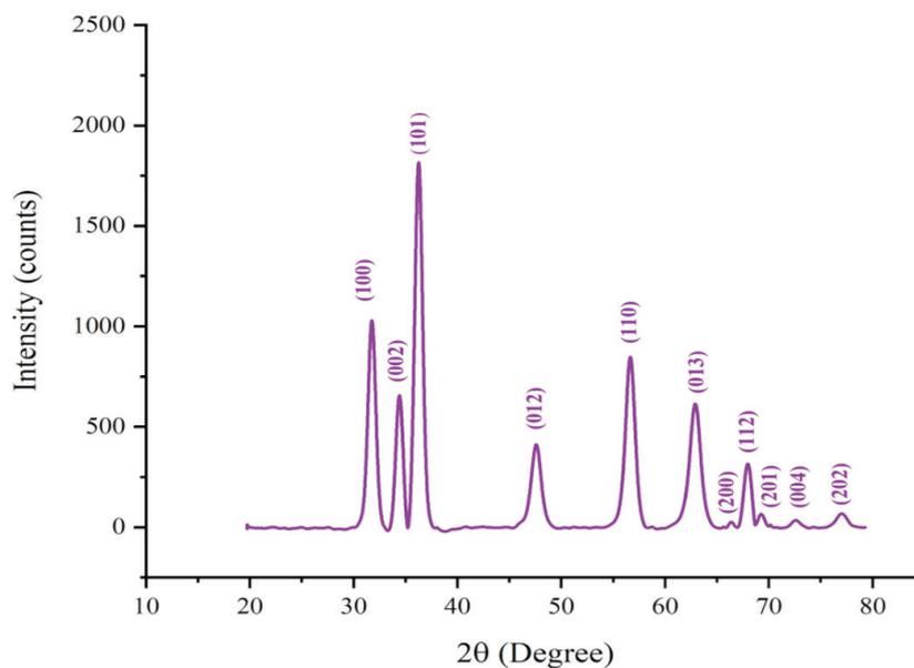
**Figure 3.** The XRD pattern of ZnO NPs.
