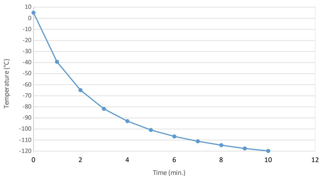
**Figure 1.** The freezing curve used to cryopreserve honey bee (*Apis mellifera* L.) sperm for all treatments. The indicated temperatures were measured in the freezing chamber above straw level by a thermometer (Hanna Inst. HI 9056)
