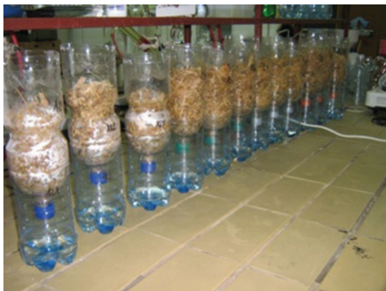
Photograph 1 and Figure 1. System for silage aerobic stability testing
