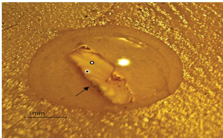
**Figure 2.** The image of the cross-section of the heated hearing stone, magnification x30 under the stereomicroscope of KRUSS, Germany). In this image, the difference between dark and light circles is shown by empty (white) and filled (black) circles, respectively. The arrow also shows the center of the rings.
