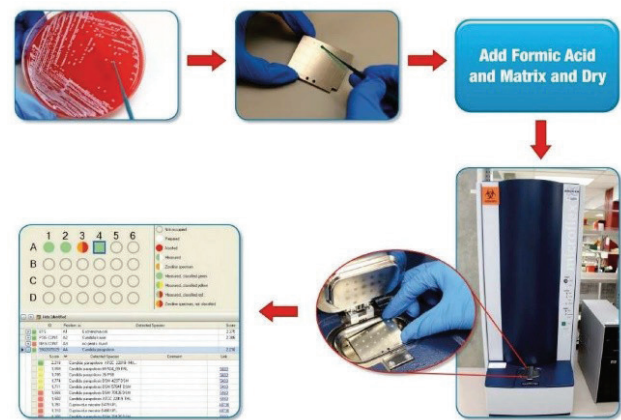
Figure 2. Matrix-assisted laser desorption/ionization time-of-flight mass spectrometry (MALDI-ToF MS) process for microfungi identification (Patel, 2015). A colony is picked from a culture plate to a spot on a MALDI-ToF MS target plate (a disposable or reusable plate with multiple spots, each of which can be used to test different colonies). For yeast applications, cells are usually treated with formic acid on the target plate and then dried. The spot is coated with 1-2 µL of matrix and dried. The plate is placed in the ionization chamber of the mass spectrometer. A mass spectrum is generated and compared by the software to a library of mass spectra, resulting in the identification of the yeast (in the example Candida parapsilosis at position A4). Used with permission from Mayo Medical Education and Research Foundation. All rights reserved.
