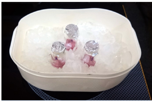
Fig 1: vials contain sheep conjugate and gold nanoparticles
