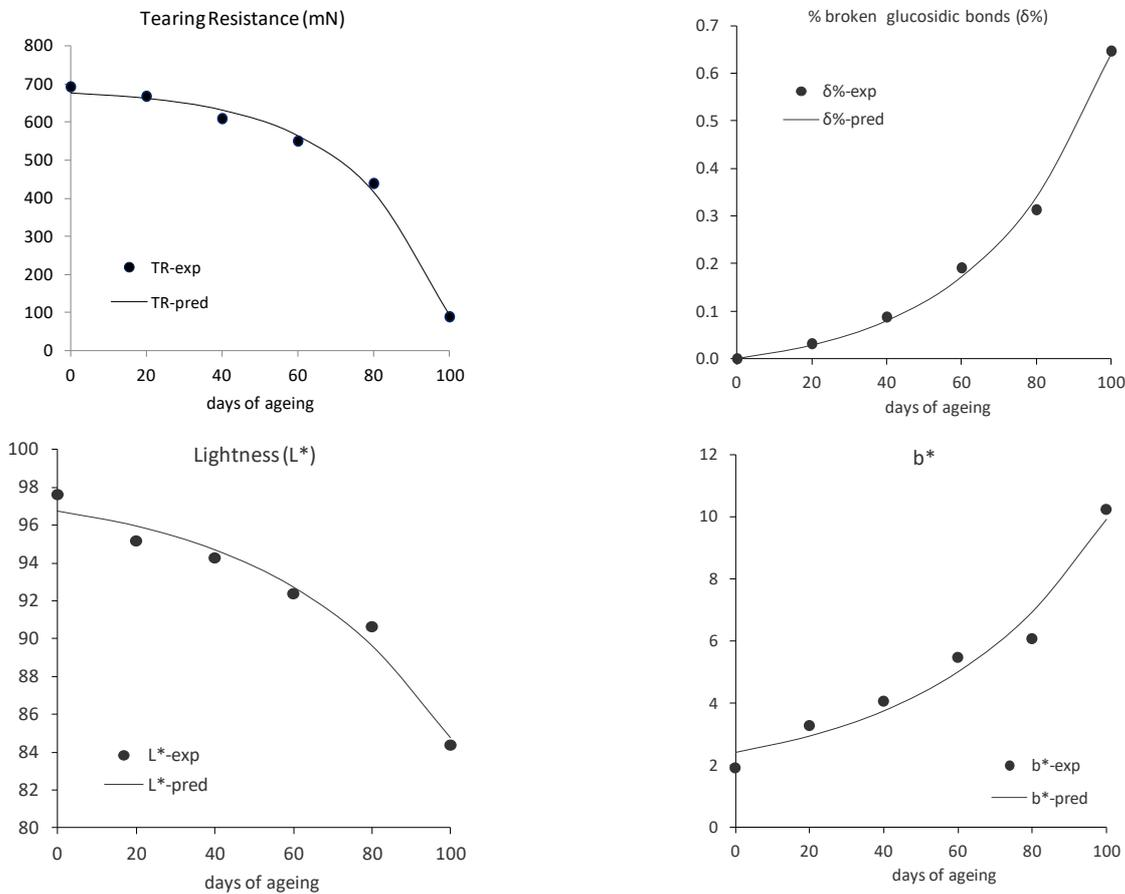
Figure 2. Plots of TR (Tearing resistance),  $\delta\%$  (percentage of broken bonds), and  $L^*$  and  $b^*$  coordinates of the CIEL\*a\*b\* color system against time of ageing. Experimental (exp, dots) and predicted (pred, lines) values.
