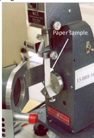
**Fig. 4.** The folding endurance tester of the General Chemical State Laboratory (G.C.S.L.) in Athens [MIT instrument type, [20 p. 27]]. The paper sample is held by two clamps. The lower clamp is movable and folds the sample to an angle of 135° in either direction. The desired stress is applied to the specimen by an adjustable spring.
