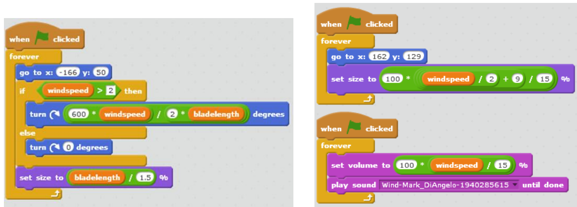
Figure 6. Programming Blocks that rotate the blades of the 3-blade turbine and produce the sound of the wind blow by simultaneously varying the size of the Wind God's head
