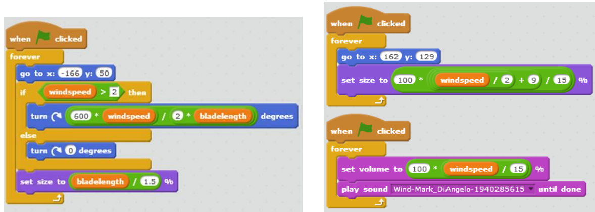
Figure 6. Programming Blocks that rotate the blades of the 3-blade turbine and produce the sound of the wind blow by simultaneously varying the size of the Wind God's head
