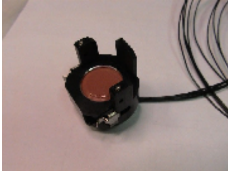
Figure 1: Tactile Motors (Courtesy of CompuTouch(WWW))
