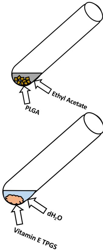
1) mix 100 mg PLGA with 1ml Ethyl Acetate (test tube I)
