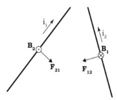
In the figure, there are two straight current-carrying conductors that are not parallel. It is clear that the forces developed between them are not opposite. Based on the vector relationship that arises from Newton's third law  $\overrightarrow{F_{21}} = -\overrightarrow{F_{12}}$ , this case seems to be incorrect. To explain this paradox, let us examine the total momentum of the system  $\overrightarrow{p_s}$ . If we assume that the bodies are in equilibrium, we have:
