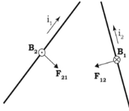
In the figure, there are two straight current-carrying conductors that are not parallel. It is clear that the forces developed between them are not opposite. Based on the vector relationship that arises from Newton's third law  $\vec{F}_{21} = -\vec{F}_{12}$ , this case seems to be incorrect. To explain this paradox, let us examine the total momentum of the system  $\vec{p}_s$ . If we assume that the bodies are in equilibrium, we have:
