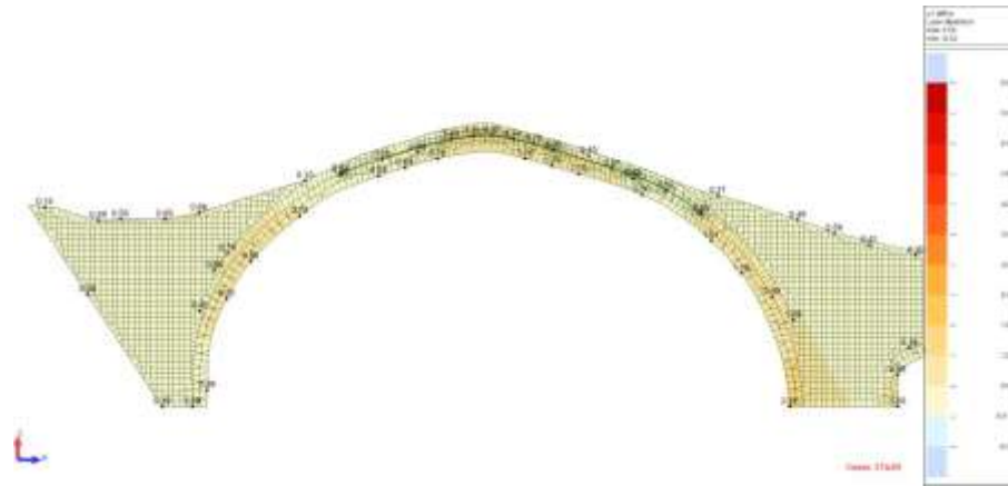
Fig. 14. Results after reinforcement: Seismic design load. Principal tensile stresses \sigma_1 stresses \sigma_1 (MPa)
