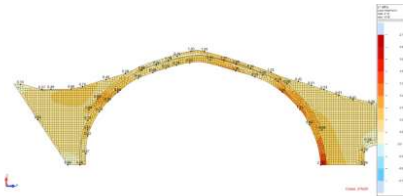
Fig. 13. Results before reinforcement: Seismic design load. Principal tensile stresses \sigma_1 (MPa)
