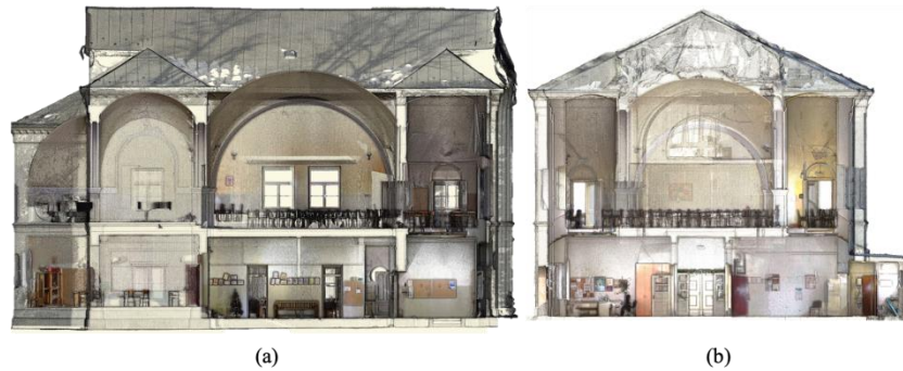
Fig. 3. Longitudinal (East-West) (a) and lateral (South-North)(b) cross-section of building acquired from 3D point cloud model after earthquake of December 2020
