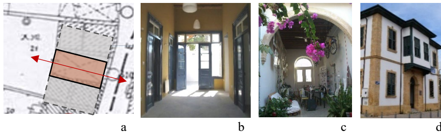
Fig. 2. a) Typical tripartite arrangement of houses with portico (highlighted in colour); b) View of a pass-through portico space – towards the courtyard; c) A portico space in the original, semi-open form – view towards the street; d) Two-storey building with tripartite arrangement and sahnisi projecting volume on the first floor.
