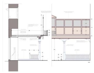
Fig. 11. Constructional details of the mezzanine
