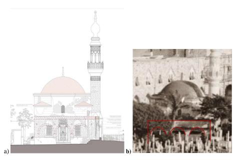
**Fig. 7.** (a) Representation of the porch's façade. (b) Photo of the Mosque in 1927, on which the porch is shown with red lines. [Reproduced from the archive of Stavros Georgallidis]
