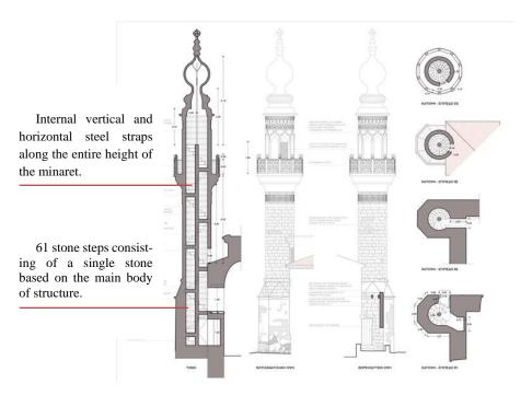
Fig. 12. Constructional details of the minaret.
