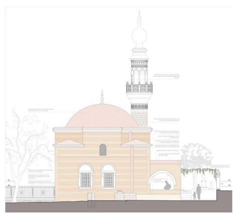
**Fig. 14.** Restoration proposal of the NE façade following the existing phase of the plastering with the horizontal zones in ceramic and ocher colors.
