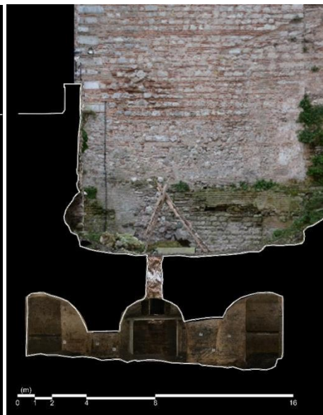
Fig. 25. Section 3-3 of the hypogeum.
