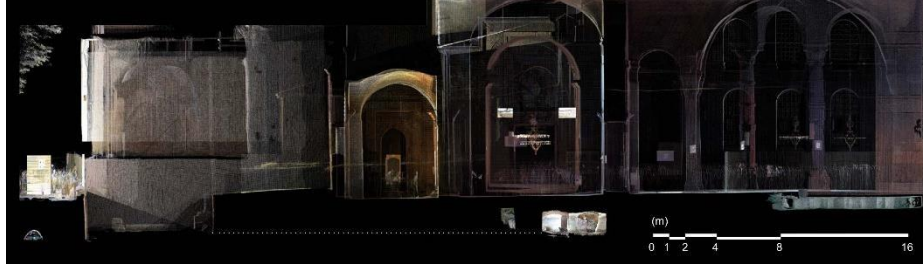
Fig. 5. Section 2-2: Northwest-southeast cross-section extending from the remains of the Theodosian portico to the northern main pier of Hagia Sophia.
