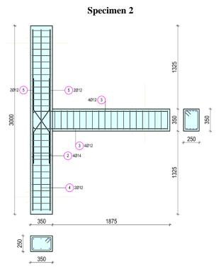
Fig. 1. Geometrical characteristics of the specimens 1 and Specimen 2
