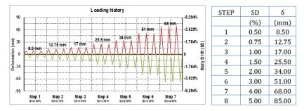
Fig. 3. Loading sequence. Eight loading steps and each step includes three full loading cycles
