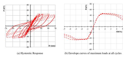
Fig. 5. Hysteretic response and load envelope of all cycles of Specimen 2
