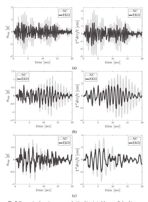
**Fig. 9.** Comparative dynamic response results (time histories) of the controlled multi-story structures with distributed EKD devices (left: top floor absolute acceleration  $a_{top}$ , right: first floor drift  $I^{st}$  *drift*), compared to the IN, for an EC8-compatible artificial accelerogram. (a) 5-story, (b) 10-story, and (c) 15-story buildings.
