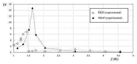
Fig. 3. Frequency response of the EKD device compared to the SDoF oscillator.
