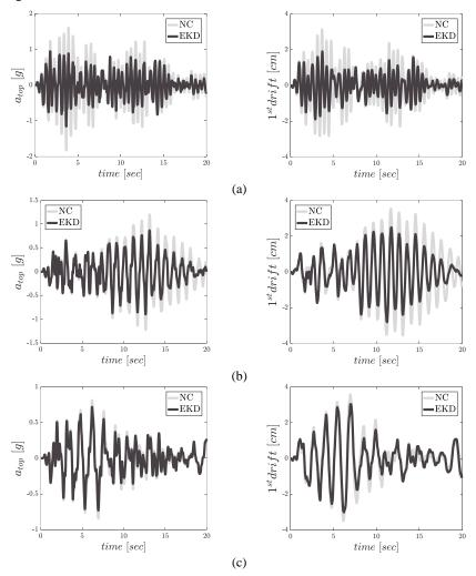
**Fig. 6.** Comparative dynamic response results (time histories) of the controlled multi-story structures with EKD device at its base (left: top floor absolute acceleration  $a_{top}$ , right: first floor drift  $I^{st}$  drift), compared to the NC, for an EC8-compatible artificial accelerogram. (a) 5-story, (b) 10-story, and (c) 15-story buildings.
