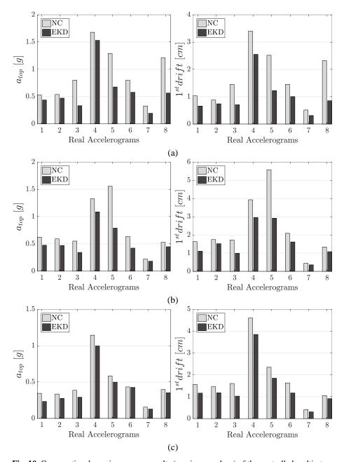
**Fig. 10.** Comparative dynamic response results (maximum values) of the controlled multi-story structures with distributed EKD devices (left: top floor absolute acceleration  $a_{top}$ , right: first floor drift  $I^{st}$  drift), compared to the IN, for all the selected real earthquake records. (a) 5-story, (b) 10-story, and (c) 15-story buildings.
