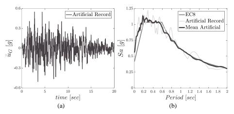
Fig. 4. (a) Artificial accelerogram, and (b) mean acceleration spectrum compared to the EC8.
