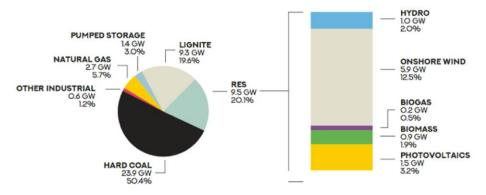
Fig. 1. Installed Capacity in the Polish system at the end of 2019 [8]
