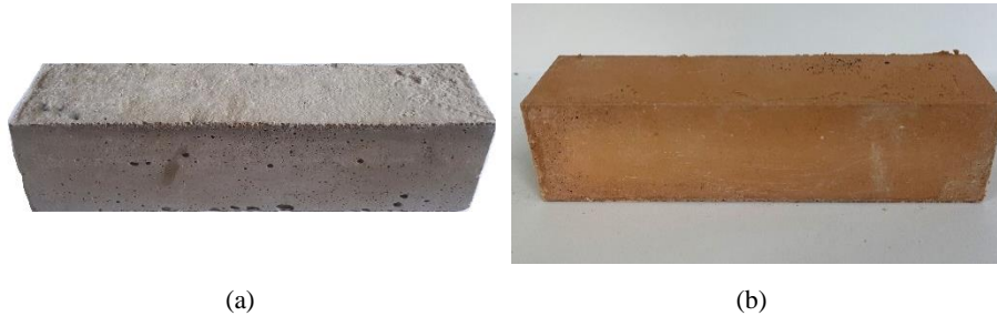
Fig. 1. Typical prism of (a) cement-based and (b) geopolymer mortar.
