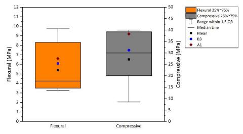
Fig. 3. Comparison between geopolymer and cement-based mortar strength.
