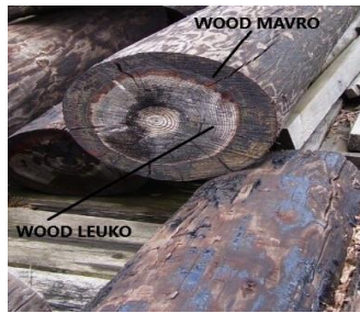
Fig. 1. Creosote-treated wood waste 70% 'mavro' (black) – 30% 'leuko' (white)
