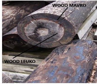
Fig. 1. Creosote-treated wood waste 70% 'mavro' (black) – 30% 'leuko' (white)
