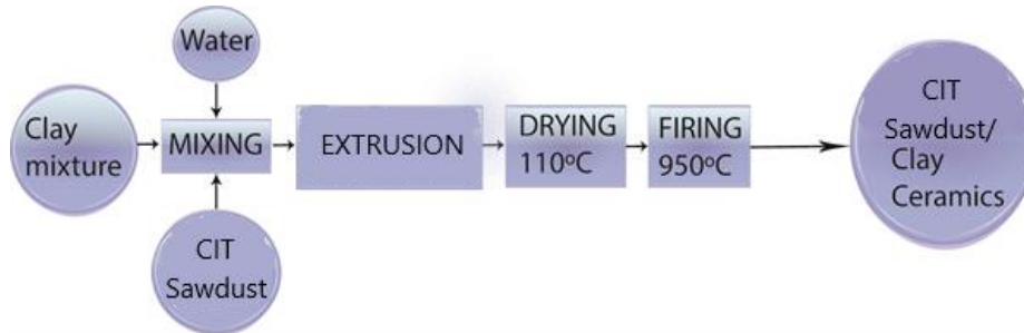
Fig. 3. A schematic representation of the process for the production of CIT sawdust/clay-based red ceramic specimens.
