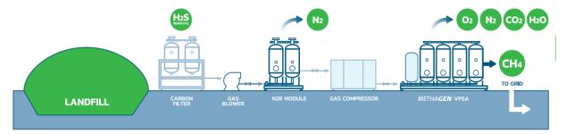
Fig. 9. METHAGEN LF system schematics for Landfill gas upgrade - SYSADVANCE
