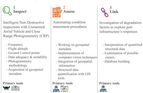
Fig. 2. The steps of building a UAV-based SDT of port concrete pavements
