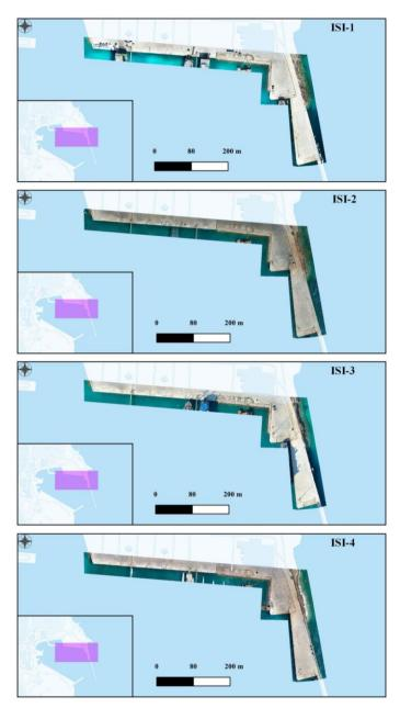
**Fig. 5.** The four orthophotos illustrating the concrete pavements of the mooring facilities of the domestic ferry and the cruise domain of the Lavrio port for the four (4) in-situ inspections: ISI-1 (2020-02-10), ISI-2 (2020-09-04), ISI-3 (2021-02-10), and ISI-4 (2021-07-09) [32]-Step 1 of Figure 2
