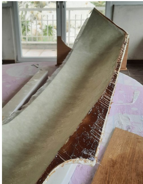
Fig. 24. Placement of polyester glue in the keel
