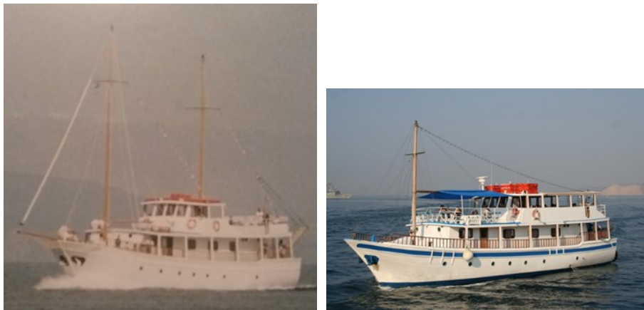
Fig. 1. The traditional yacht Kostantis (a) between 1999 and 2001, (b) after retrofitting and removal of the masts
