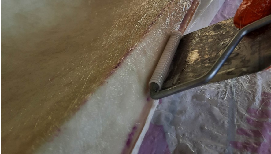
Fig. 23. Removal of trapped air bubbles
