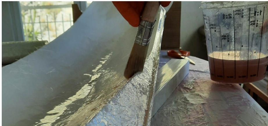
Fig. 22. Coating of polyester resin on the surface of the mold
