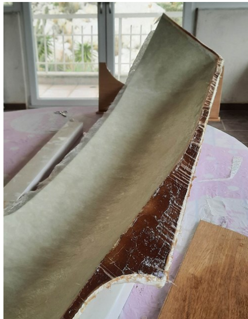
Fig. 24. Placement of polyester glue in the keel
