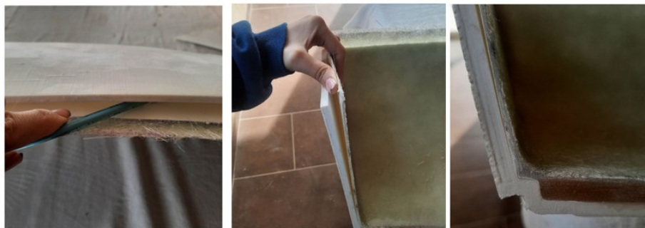
Fig. 26. The process of removing the GRP hull model from the mold
