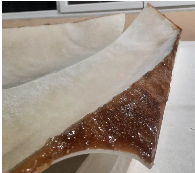
Fig. 28. Application of polyester glue to join the two parts of the GRP model
