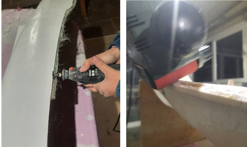
Fig. 27. Removal of excess polyester and glass fabric with rotary multi-tool and roller sander
