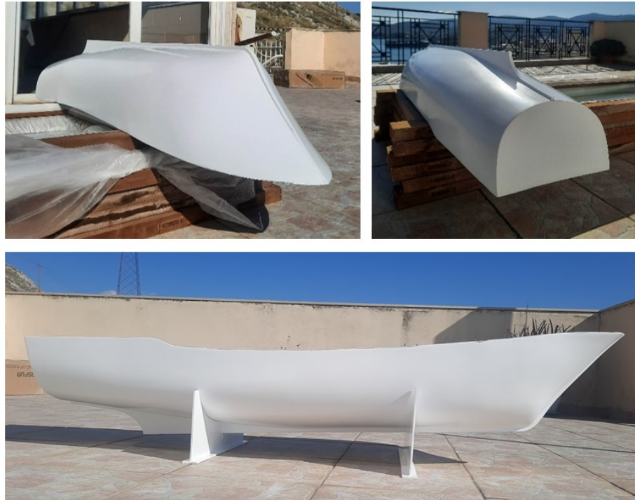
Fig. 30. Bow (top left), stern (top right) and right view (bottom) of the GRP hull model
