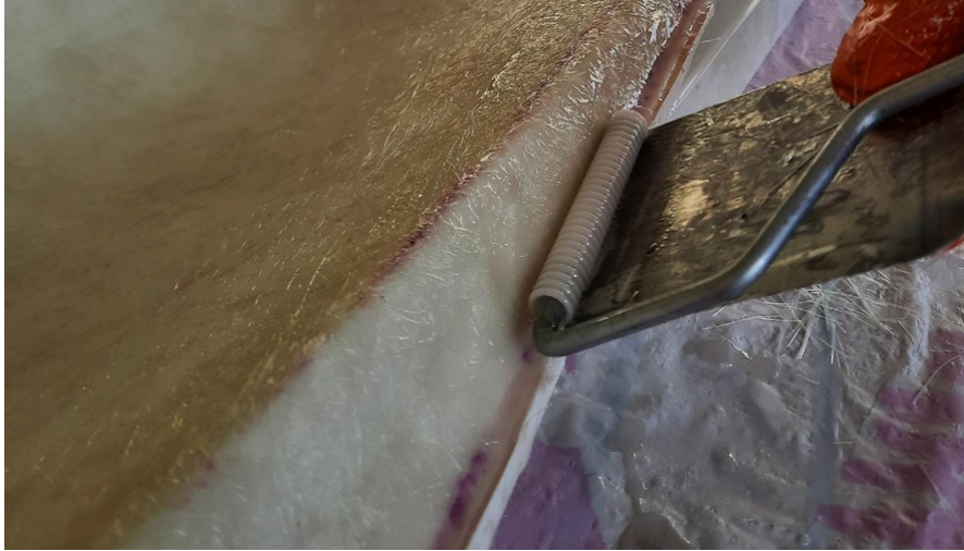
Fig. 23. Removal of trapped air bubbles
