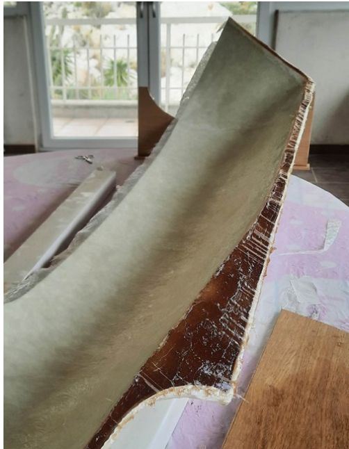
Fig. 24. Placement of polyester glue in the keel
