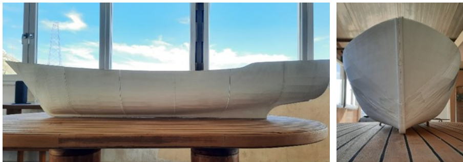
Fig. 20. The 3D printed hull prototype of Kostantis, built to 1:15 scale
