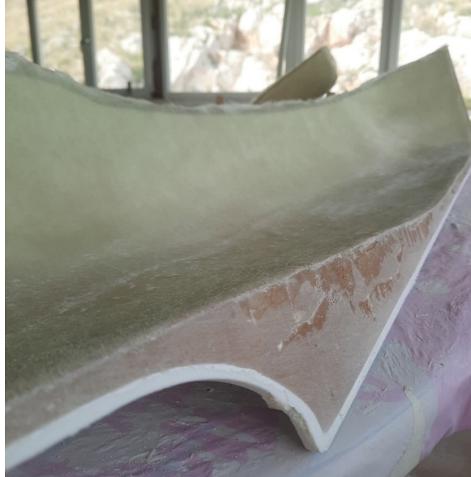
Fig. 25. The GRP hull model 24 hours after hand lay-up application
