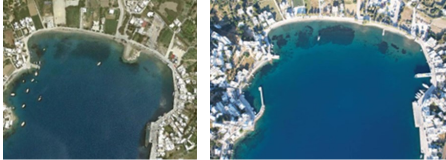
Photos 9. & 10. Satellite and drone taken photos of Katapola bay, before (9) and after (10) the construction of the fishing shelter (formed on the left side of Katapola bay). The artificial pier's materials have been incorporated into shelter's breakwater. The beach has been already returned to its initial condition
