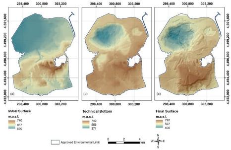
**Fig. 2.** Digital Elevation Maps of three different phases in Amyntaion mines: (a) initial surface before the excavation works, (b) the technical bottom declaring the excavation areas, and (c) the final post-mining surface
