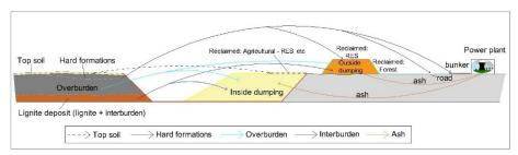
Fig. 3. Spatial representation of waste management in a surface coal mine
