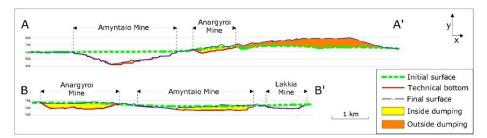
Fig. 11. Cross sections A-A' and B-B' showing the mining sequence
