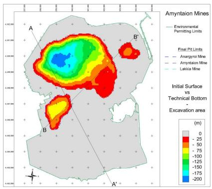
Fig. 8. Excavation sites of the Amyntaion mines
