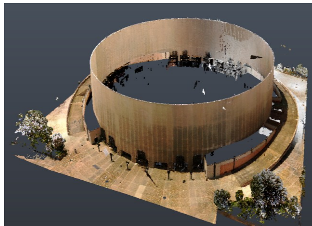
Fig. 6. The 3D point cloud of the Frank Erwin Center, processed and visualized using Autodesk Recap
