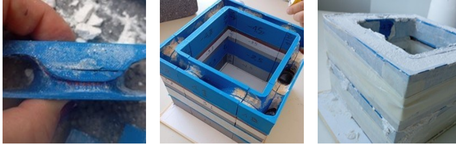
Fig. 11. Assembly and Casting Procedure. (left) view of the interior of the printed mold, (center) the four layers assembled, (left) casting procedure
