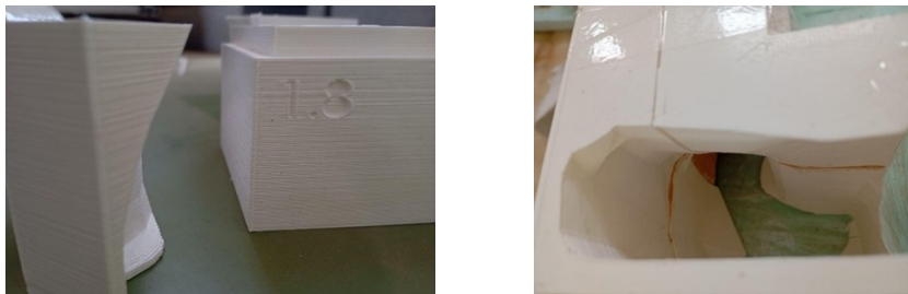
Fig. 14. Assembly and Preparation Procedure. (left) mold pieces with number engravings (right) the assembled pieces
