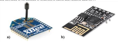
Fig. 6. (a) XBee RF module, (b) ESP8266 WiFi module.
