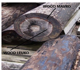
Fig. 1. Creosote-treated wood waste 70% 'mavro' (black) – 30% 'leuko' (white)
