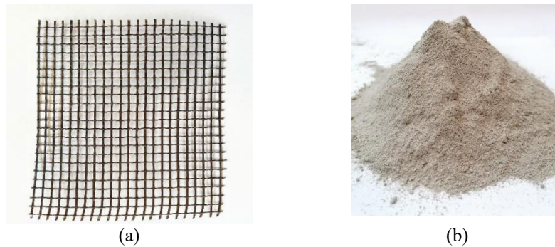
Fig. 2. (a) Basalt textile used for confinement (b) Cementitious mortar
