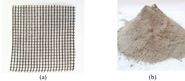
Fig. 2. (a) Basalt textile used for confinement (b) Cementitious mortar
