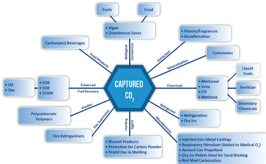
Figure 1 Classification of CO 2 utilisation options (Provided by the US Department of Energy's National Energy Technology Laboratory)
