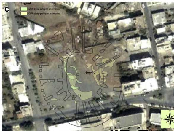
Fig. 13. Diagrammatic interpretation of strong GPR reflections and high resistivity anomalies of the area where the amphitheater of Hierapytna is located (after Papadopoulos et al. 2012, 1971 fig. 13c). Reproduced with permission of A. Sarris.
