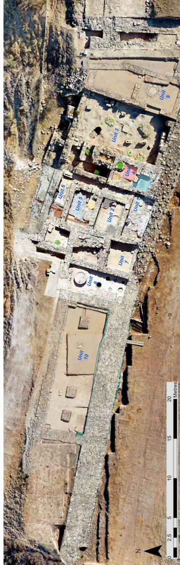
Fig. 6. True orthophoto mosaic over the Hadjiabdoullah Workshop Complex showing Units 1-10; generated from photogrammetric structure from motion (SfM) processing of high-resolution low altitude nadir and oblique drone images. Drafted by A. Agapiou (©PULP).
